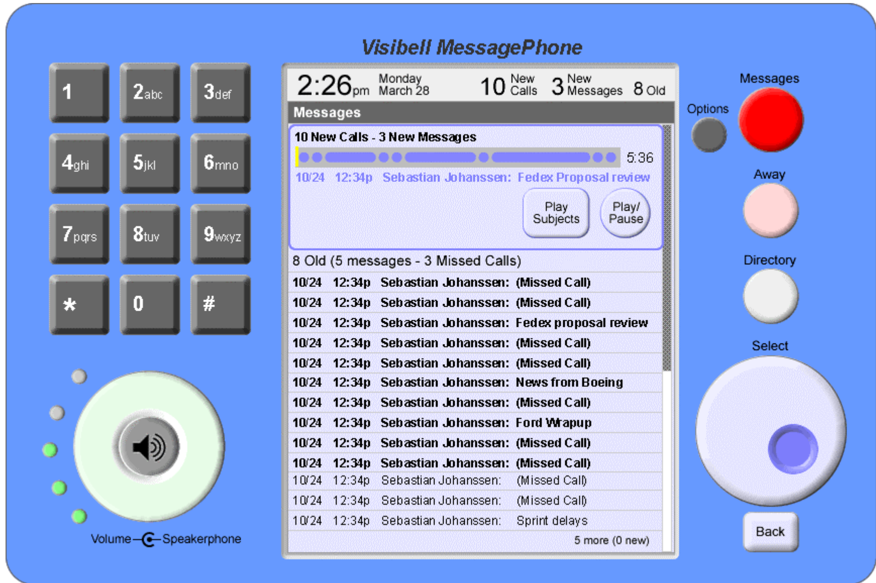
Physical layout of the face of MessagePhone
